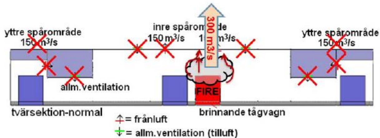
Figure 44 Centralen: Optimized smoke extraction concept.
